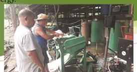
This study will compare the performance of Electric Creping Mill and Rice Hull Gasifier Powered Creping Mill.
